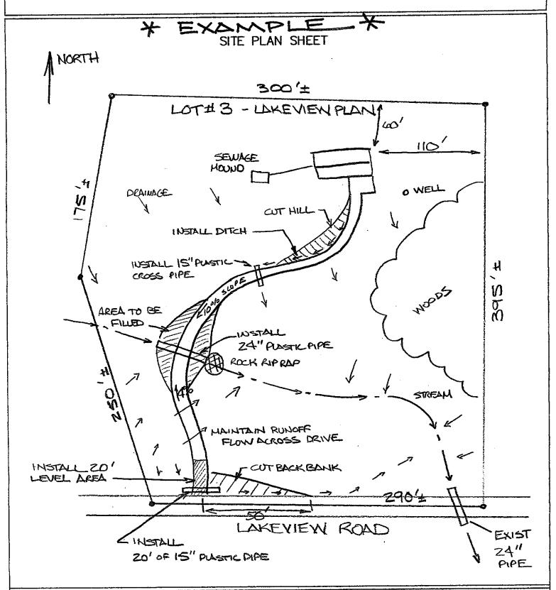
Provide a drawing of the complete driveway configuration. Show existing and proposed drainage patterns (flow arrows), drainage structures, stream crossings, areas to be cut and filled, the proposed driveway grades, and locations of other planned facilities (house, sewage system, etc)
